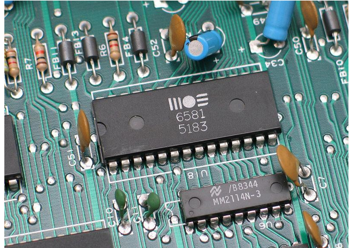
A sound chip from a 1980's Commodore 64 connected to the motherboard
